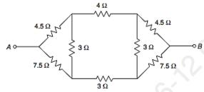
**B**) Replace the circuit between A and B in Figure with a voltage source in series with a single resistor.
